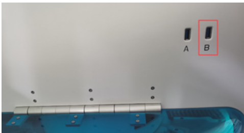
Figure 17: USB port B highlighted in red where the USB drive needs to be inserted to update the firmware on the CleanXtract 96.
