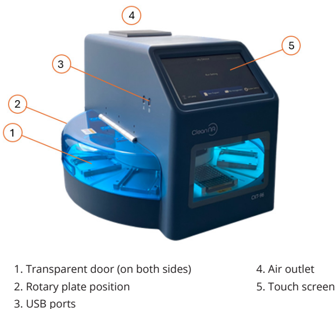
Figure 2: Overview of the different components of the CleanXtract 96.
