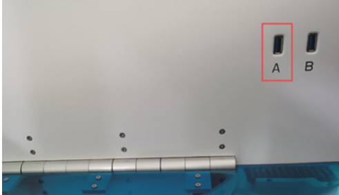
Figure 16: USB port A highlighted in red where the USB drive needs to be inserted to update the software on the CleanXtract 96.
