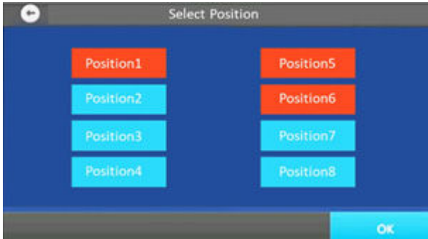
Figure 2: Select Position interface of the CleanXtract 96 with heated positions indicated in red.
